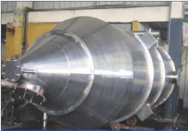
Bagfilter for drier on pharmaceutical powder
