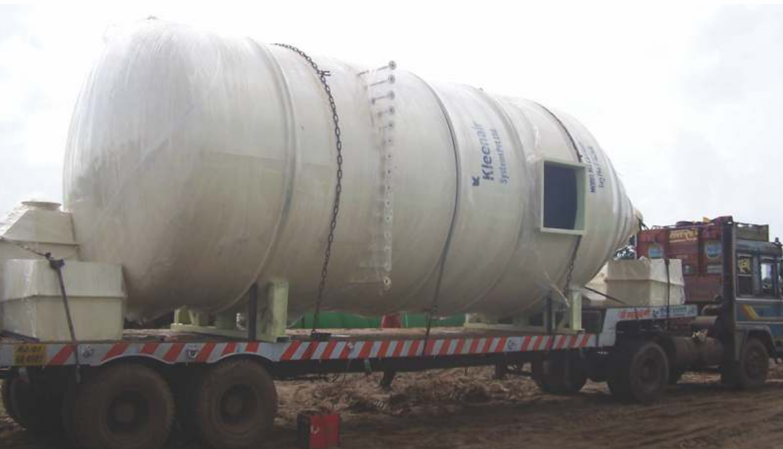
Baghouse for product collection from rotary kiln handling explosive dust
