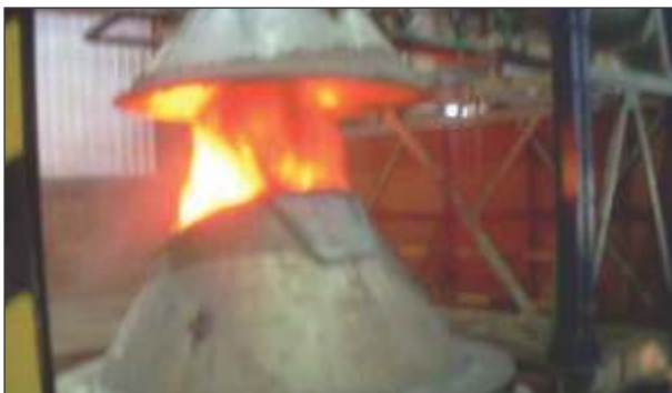
Suction of fumes through AOD when GCP in operation
